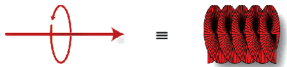
FIGURE 1. Interaction between electric (linear) and magnetic (circular) transition dipoles leading to a helix that can interact distinctly with the two circularly polarized components comprising plane polarized light.
